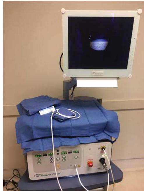
**Fig. 1** Current ophthalmic endoscopy surgical systems consist of a multifunction microendoscope and a wheeled cart housing a central console (base unit) and a two-dimensional video monitor. The base unit provides an illumination source (usually xenon), a high-resolution video camera, interfaces for microendoscope fiberoptic cabling, and connections for video output to remote monitors. It can also incorporate a photocoagulation laser source and equipment for digital image enhancement
